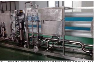
treatment equipment for medicine by using its own advantages and long-term practice. The world's most advanced reverse osmosis membrane elements, pressure vessels and high-pressure pumps are adopted, together with reasonable and efficient pre-treatment equipment and post-treatment fine desalination equipment. The configuration of the equipment and the quality of product water fully comply with GMP standards.
